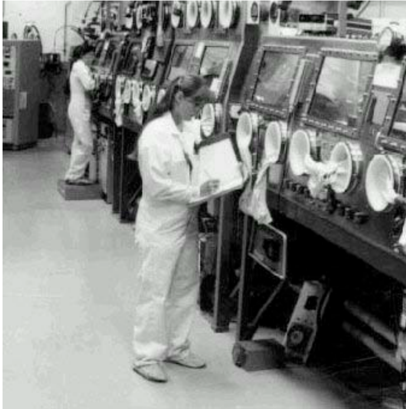
Figure 4.5: Workers at a line of gloveboxes. Plutonium is moved from box to box along an assembly line.
