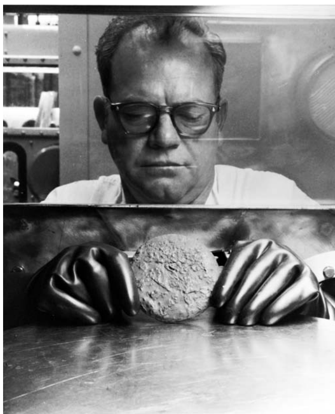
Figure 4.4: Worker on the outside of a glovebox looking in where, with his hands inserted in lead-lined gloves, he holds a plutonium “puck” that will be shaped into a pit.
