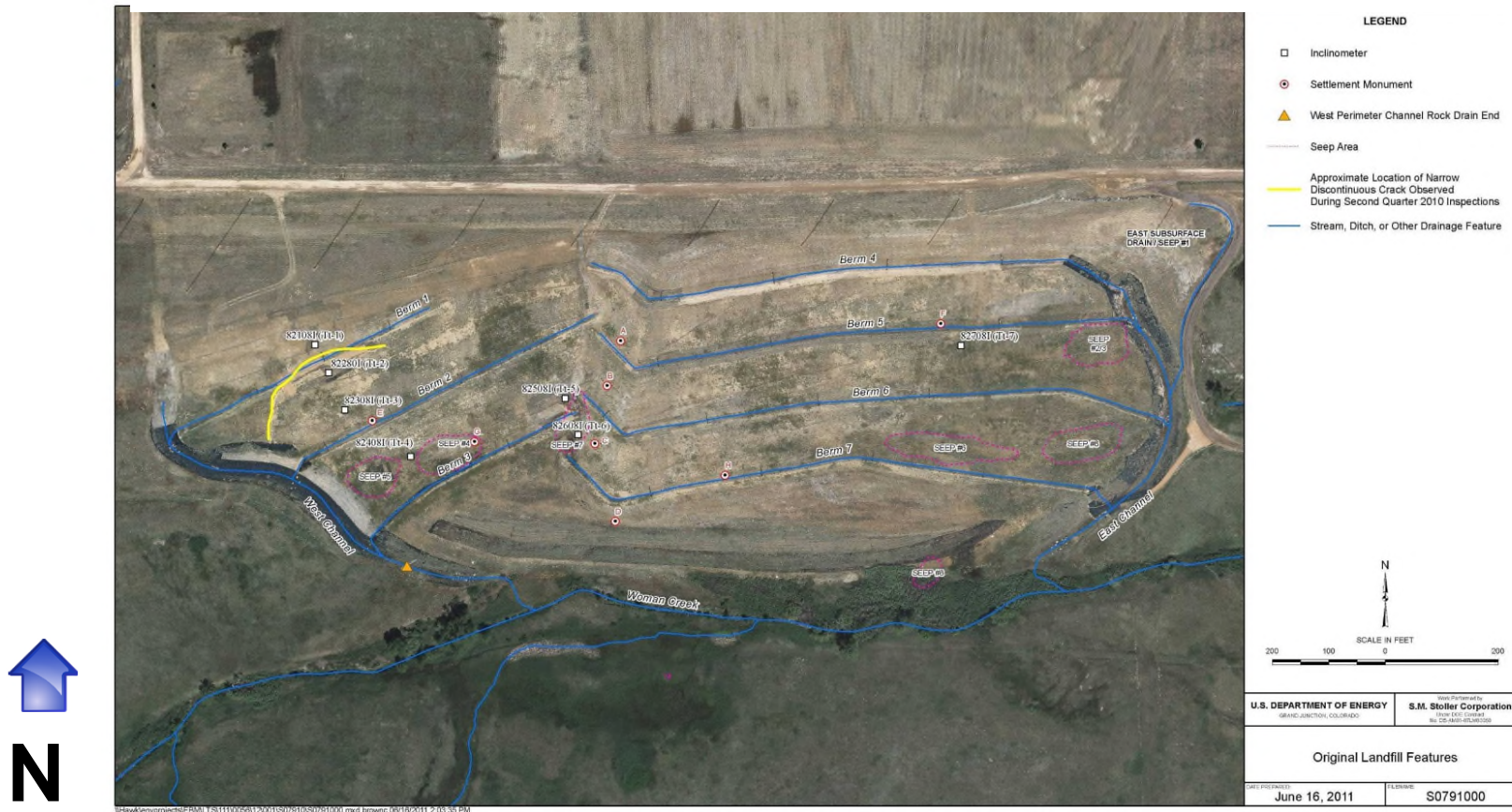
Figure 1. Original Landfill Observed Surface Cracking Location and Inclinator Locations
